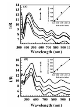
Figure 4. Inverse of the reflectivity (1/R) spectra of Ag-NP/SiO<sub>2</sub>NWs A) and Au-NP/ SiO<sub>2</sub>NWs B) immersed in solvents with different refractive indices (RIs) as follows: (a) methanol (n = 1.329), (b) acetone (n = 1.359), (c) tetrahydrofuran (n = 1.394), and (d) toluene (n = 1.496). In the insets there are the dependencies of the plasmonic wavelengths on the RIs.
