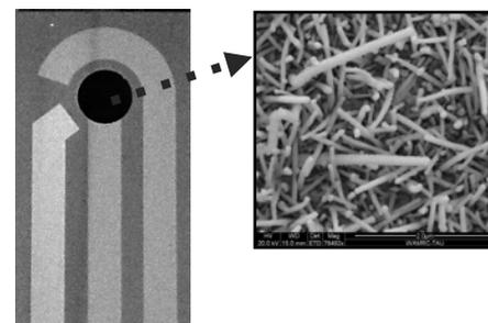
Figure 1. Electrochemical sensor with Au covered SiNWs as working electrode, a counter electrode made of gold and a reference electrode made of Ag
