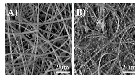
Figure 3. SEM images of SiO<sub>2</sub> NWs with Au NPs A) and Ag NPs B). Both samples were obtained with a metal coverage of 12 nm and an annealing temperature of 900 °C.
