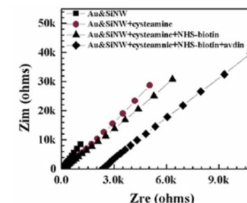
Figure 2. Nyquist plot of the electrochemical SiNW based sensor following modification with Cysteamine, Cysteamine+NHS-Biotin, and Cysteamine+NHS-Biotin+Avidin (1 μM).
