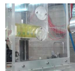
Figure 1. Apparatus for irradiating cell containing cuvettes in sequence.
