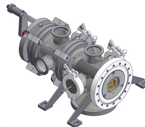
Figure 1b (right). The non-commercial ESI source at the CNR-ISM, Montelibretti, made of a heated capillary and a octupole ion guide [Design from Aarhus University].
