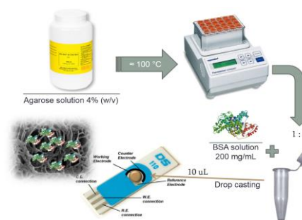
Figure 1. Probe functionalization procedure.
