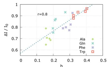
Figure 3. Pore clogging estimator  $b$  Vs measured current blockage  $\Delta I / I_0$ . Linear regression curve is reported in dashed blue, Pearson correlation coefficient  $r = 0.8$ .
