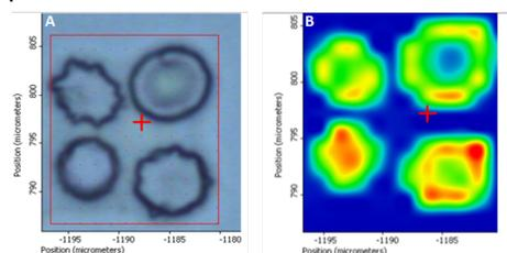
Figure 1. Optical (A) and spectral (B) maps collected with the Raman microscope on one of the smears. (A) map demonstrates the ability of the technique to distinguish between different RBC morphologies. At each point of the spectral map is associated a full range spectrum: (B) presents one of its possible visualization obtained by using 1585
