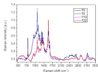
Figure 2. Mean Raman spectra for the 4 ageing times T0, T6, T13 and T22 as calculated by considering all the corresponding mean cell spectra..
