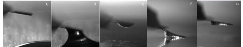
Figure 2: selected snapshots taken during the polymeric wedge formation. A) A fabricated Si 3 N 4 cantilever is approached to a UV-curable resin droplet. B) the cantilever is wet by the resin and C) withdrawn. F) the cantilever is pressed against a non-interacting flat surface, and cured in situ. G) the formed cantilever with a polymeric wedge is ready.
